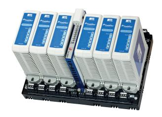
The 919x-FP module provides galvanic isolation between the 24V DC input power and the fieldbus segments, as required by the IEC61158-2 fieldbus standard and the Fieldbus Foundation™ FF-831 validation test for power supplies. There is also galvanic isolation between the fieldbus segments, thereby preventing multiple segment failures due to ground faults on more than one segment.
