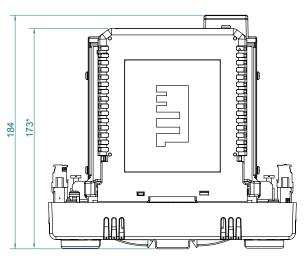
\* This dimension applies if the F809F-Plus diagnostic module is not used.
